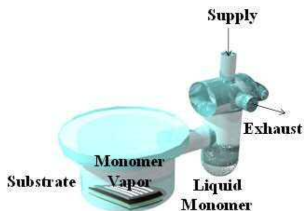
Fig. 1. H-shaped reactor for vapor-phase assisted surface polymerization.
