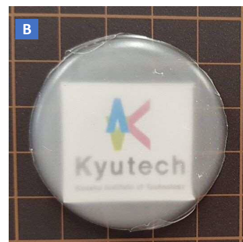
Figure 2: A) Silicone, B) Silicone/NC Composite (2.0mm Thickness)
