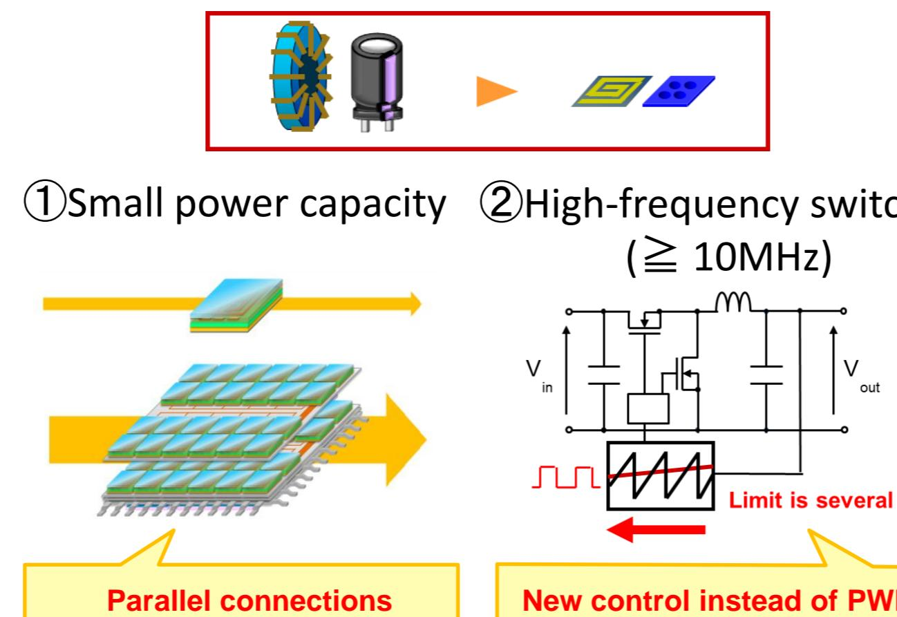
✓ Power SoC based on parallel connections of many dc-dc converters
