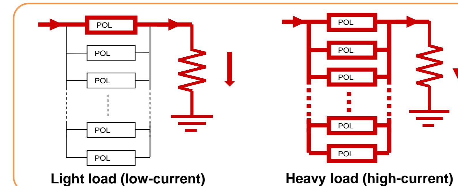
Switching number N in response to output current
